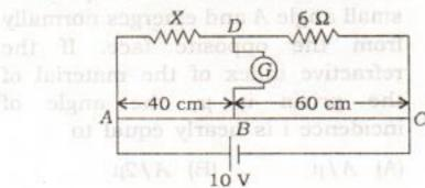
The metre bridge wire has a resistance of  $0.1 \Omega/cm$ . The current drawn from battery of negligible resistance is
